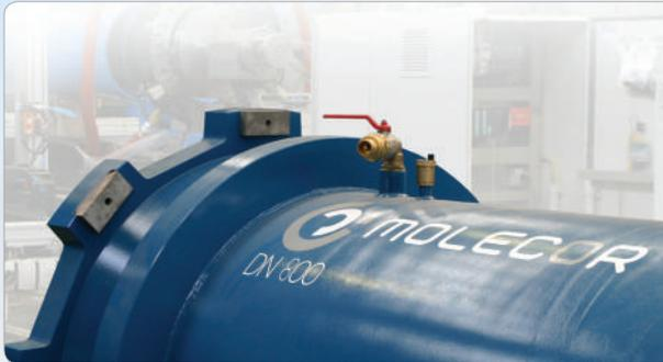
The biggest PVC-O pipe has been developed by Molecor, a pipe of DN 800 (30").
